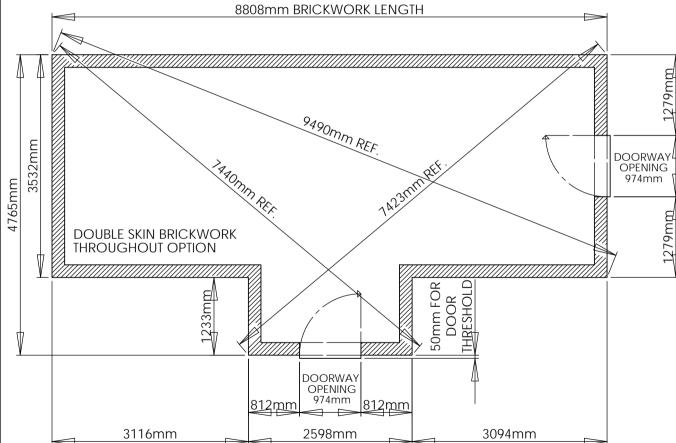
NOTE: RETURN BRICKWORK EITHER SIDE OF PORCH IS 22mm DIFFERENT, THEY ARE NOT EQUAL.
